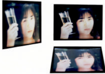
Fig. 1. Casio's 2.5-inch diagonal 832x230 active matrix TLAF prototype. The drive voltage is \pm 2.5V ; time to scan one line, 60\mu s ; and contrast ratio over 300. The upper right is a front view. The other images show no gray scale inversion nor color change even when the viewing angle is as in the lower right [6]. Courtesy T.Yoshida: tyoshida@drd.hlb.casio.co.jp
