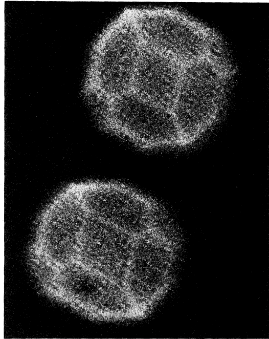
FIG. 1. Photomicrograph of monocrystals of BPI (in equilibrium with isotropic liquid) in monochromatic illumination. The crystal habit indicates cubic point symmetry, O .
